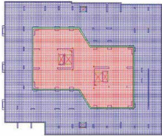
Project Outline: Blue represents the not isolated area corresponding to near 3.700 m 2 of underground, while red refers to the isolated area of 1.400 m 2 (base plate where the devices will be placed). Green refers to the 50 cm expansion left to avoid collision between the two buildings. Courtesy of René Lagos Engineers.
