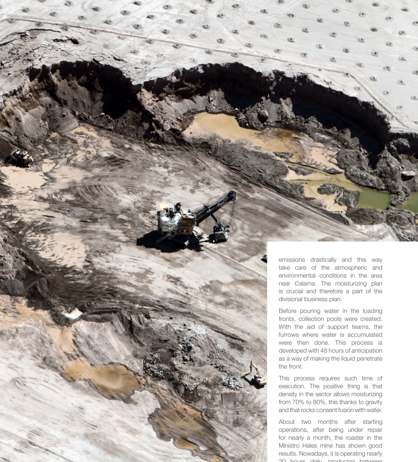
End of pre-stripping, 228 million tons of sterile material had to be removed, the equivalent of 70 times the Santa Lucía Hill in Santiago. Courtesy of Codelco.
