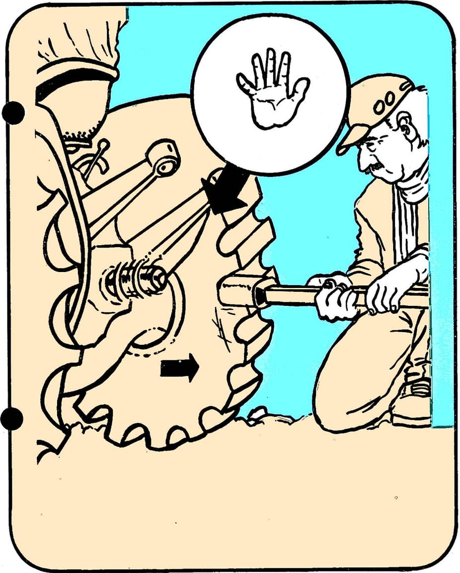
NO ACOPLA CON EJE EN MOVIMIENTO.
